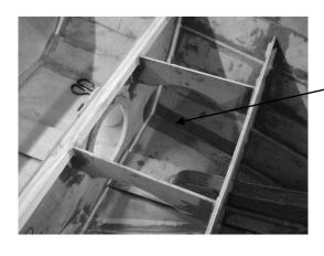
Step A – apply epoxy either side of the joint and on the bulkhead at each end by a distance equal to the width of the tape.
