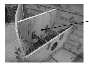
Draw a pencil line between the horizontal slots. Insert a saw in one of the slots and saw along the line. The saw cut should be level with the bottom of the slots.
